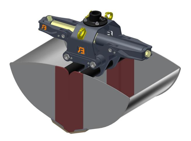
The KBX is a grab for normal excavation work. The large spread when the grab is open makes this type very suitable for loading and unloading bulk materials such as sand, powder and gravel. Standard equipped with a reinforced cylinder, which means that the grab has a very good capability to penetrate. Standard equipped with a double-walled cylinder with 2 non-return valves built into the cylinder.
